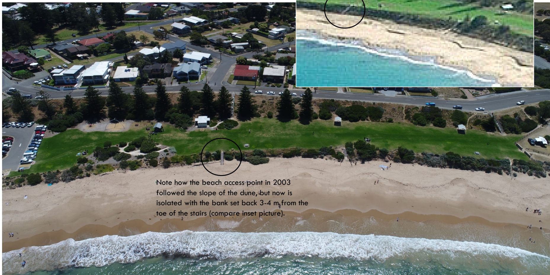
Figure 41 and 42: Comparison between backshore profiles of 2003 and 2018, DEW, 2003.
