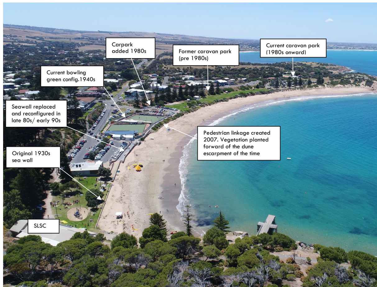
Figure 11: Horseshoe Bay in its modern form (2018). (Compare tidal lines and seaweed lines to Figure 8)
