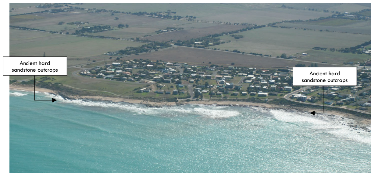
Figure 9: Location of ancient sandstone outcrops that dissipate wave energy upon the coast.
