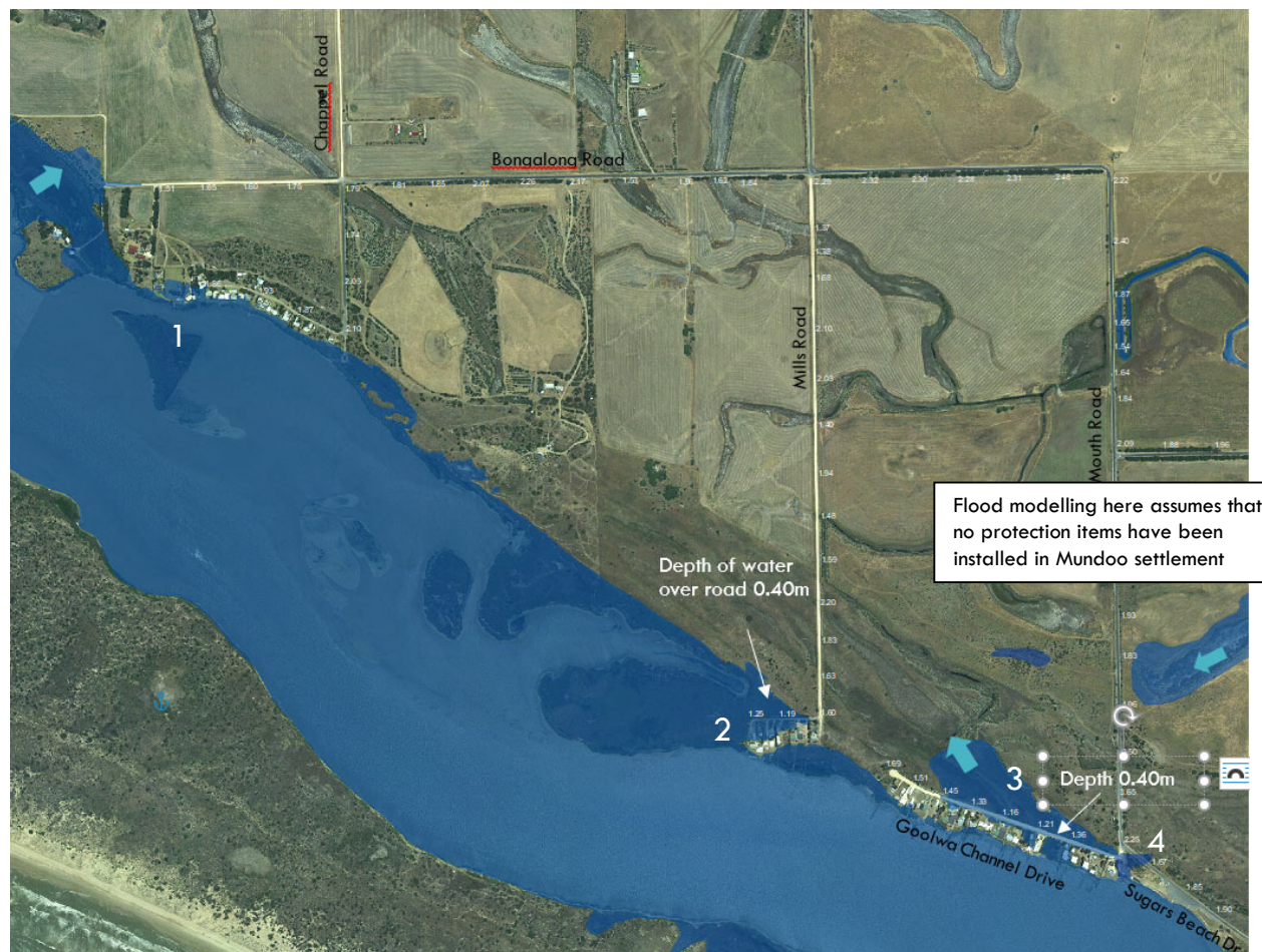
Figure 47 Modelling indicates that main access roads to the settlements situated on Goolwa Channel are not vulnerable to flooding in the current 1 in 100-year sea-flood event but four locations within settlements are vulnerable.
