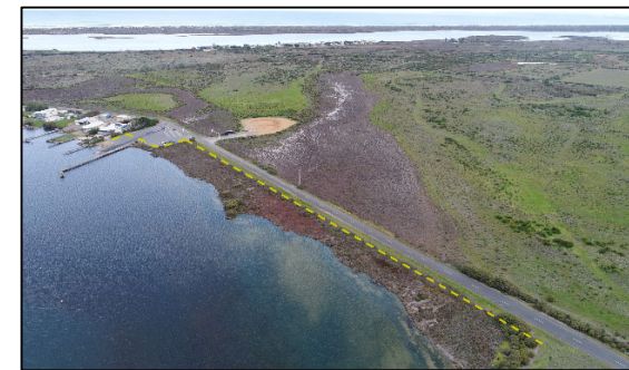
Figures 30-32 Low height levees at the northern and southern ends of the settlement would prevent water from flowing around the back of the settlement. A protection strategy would also need to be employed for privately held allotments to prevent water flowing through the settlement from the channel.
