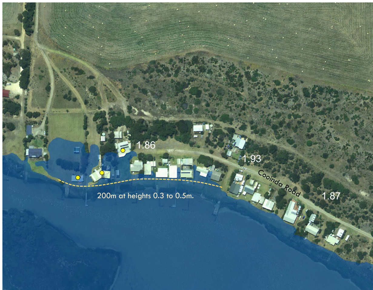
Figure 48 Modelling indicates that internal access to Cooinda Road settlement is not at risk in current 1 in 100-year sea flood event but some shack sites are vulnerable to flooding.
