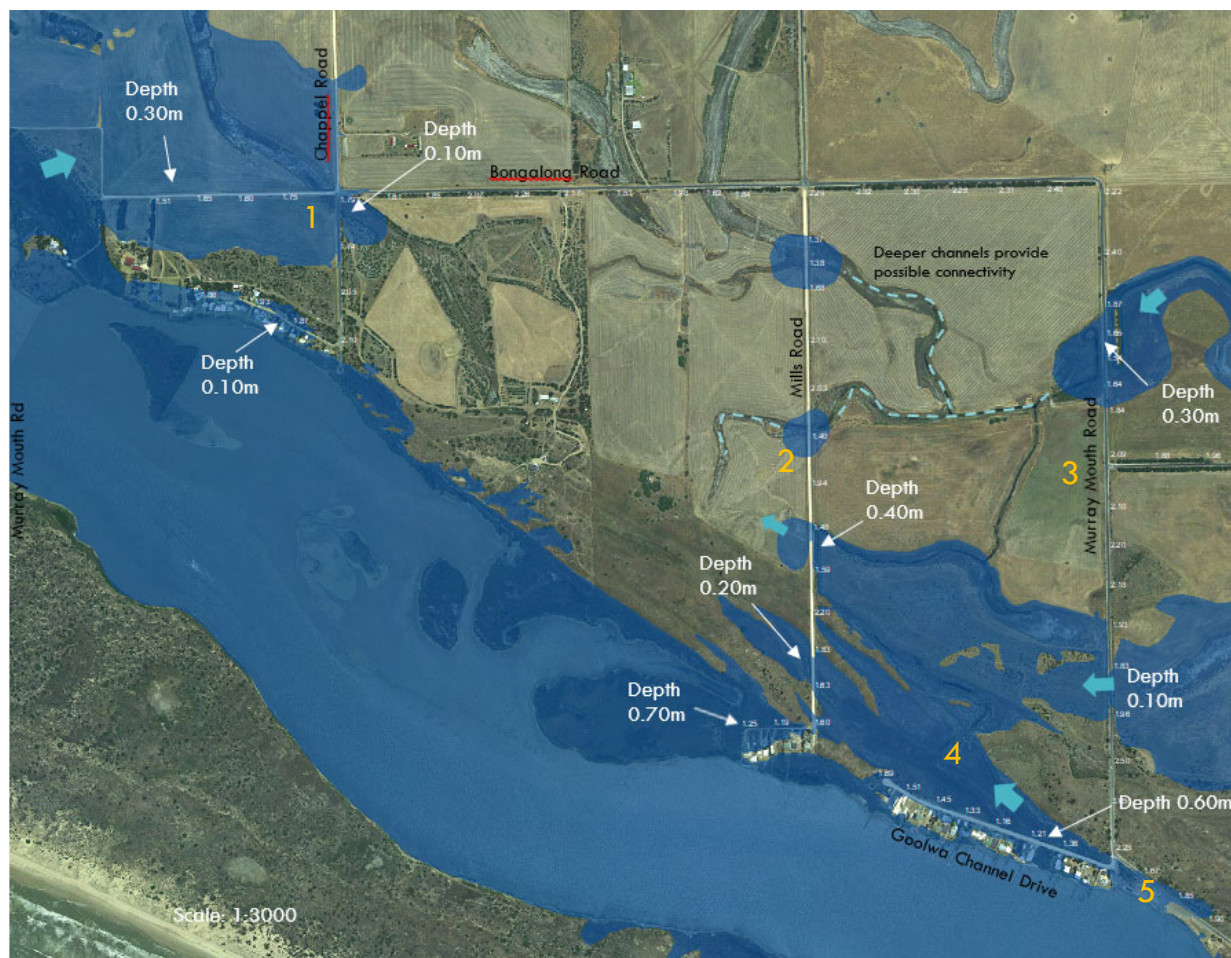
Figure 54: Main access roads and areas of settlements where scenario mapping demonstrates vulnerability to the 2050 1 in 100 ARI event.
