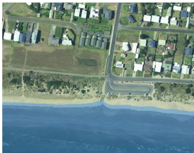
Left: Note the scouring from storm water outflow (DEM 2018). Impacts from storm effects will be greater in locations where the beach has been lowered. Sea level rise will exacerbate the problem.
