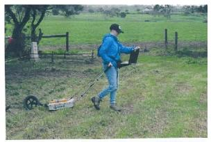
The Mala X3M Ground Penetrating Radar system used for this survey.
