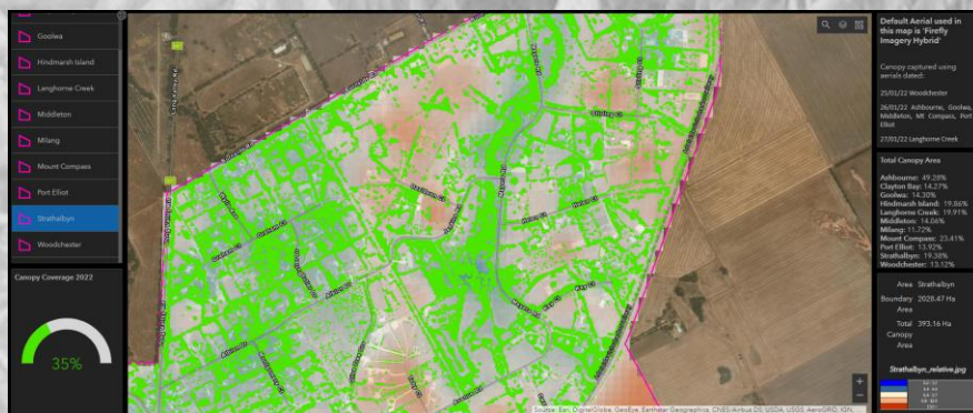
Sample image from Strathalbyn: canopy cover determined by AI with an overlay of geospatially linked thermal image demonstrating the relationship between canopy and radiant temperature
