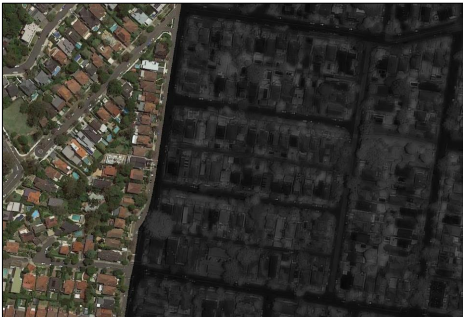
Sample of an area showing Pleiades' Near-Infrared band (right side, in grayscale), next to Google Sat aerial imagery (left side, colour image).
